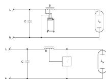
Scheda tecnica Balastro Philips HID-HighPower BSN 1000 L78 230/240V 50Hz
