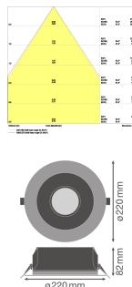
**Scheda tecnica Ledvance Downlight LED Performance DN195 21W 2520lm 65D - 840 Bianco Freddo | 220mm - IP54**
